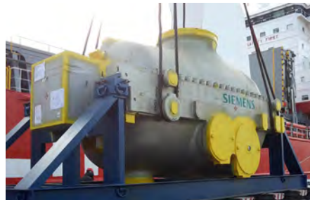
220 tons Siemens Steam Turbine on 16 wheels trailer
