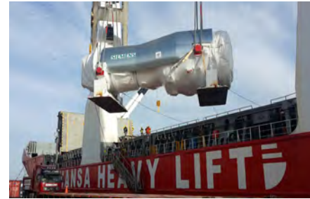
500 tons Siemens Gas Turbine
