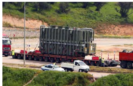
Heaviest transformer (363 tons) transport for natural gas cycling plant
