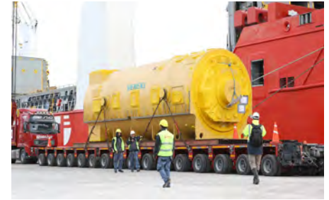
460 tons Siemens Generator on 22 wheels Goldhofer trailer
